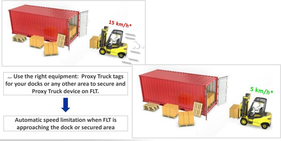
\* Speeds are modified by an action on FLT variator or Canbus. High and slow speeds are defined by the client.
