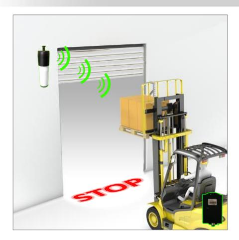
... Use the right equipment: Proxy tags on gate and Proxy device with fork height detection on the FLT ...
