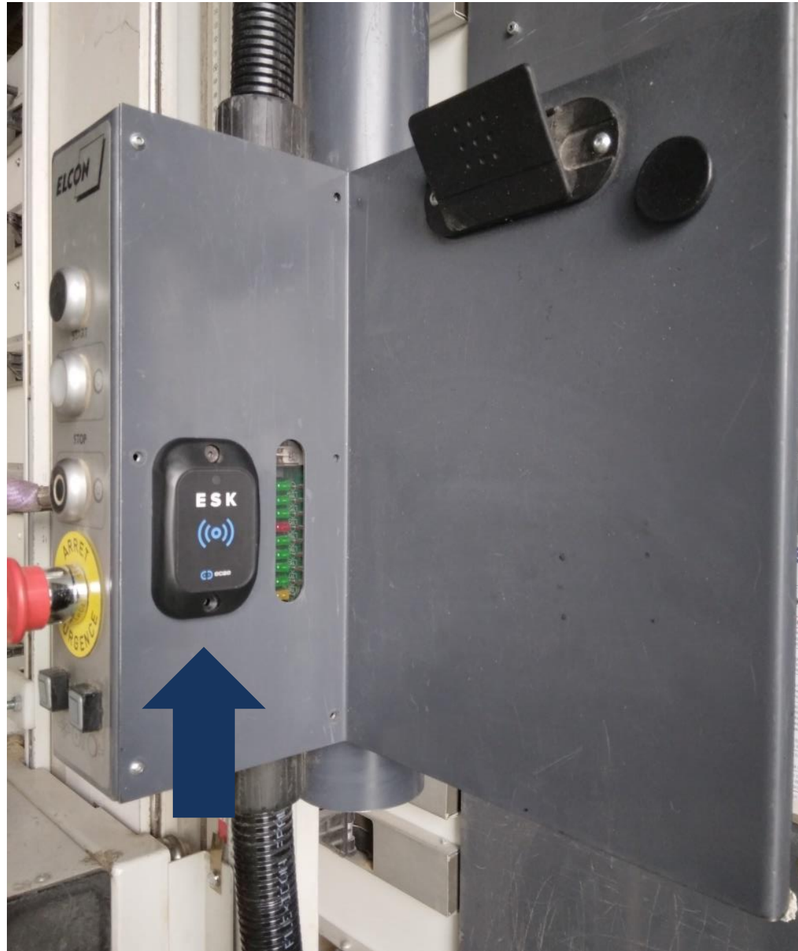
Badge reader installed on the front of the saw for user identification.
